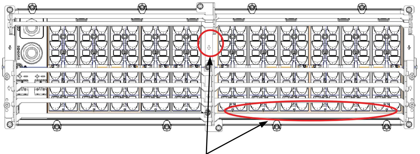
Louvre arrow in the same direction like the LED module arrow for positioning
